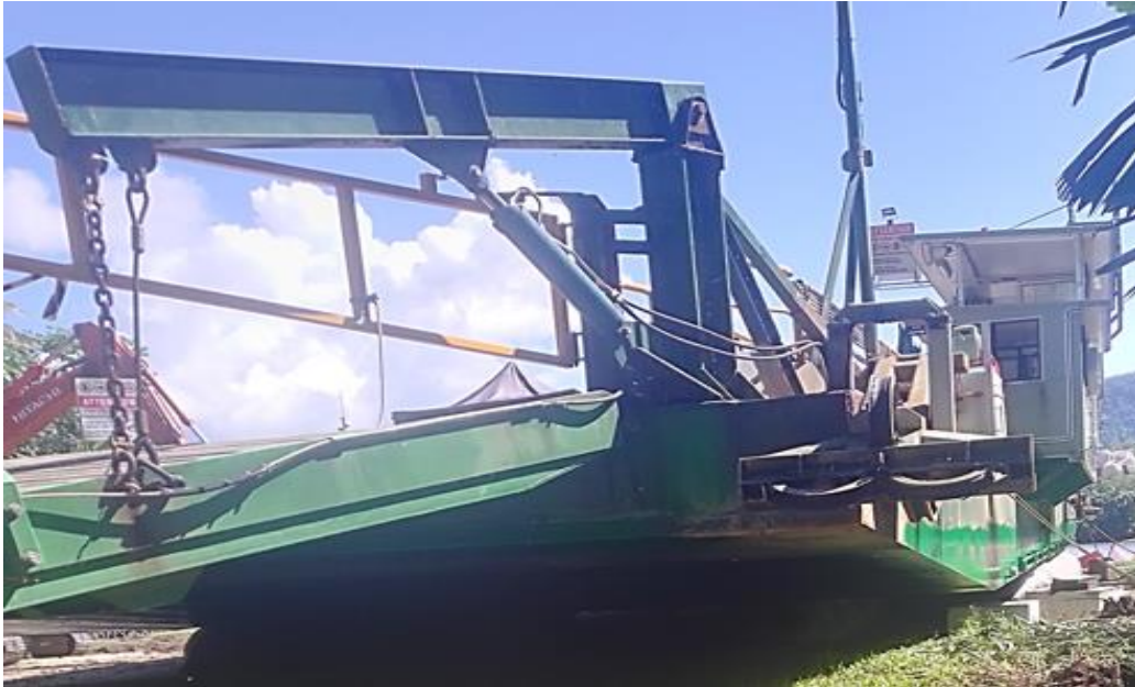
Image: Davit arm prior to modifications
