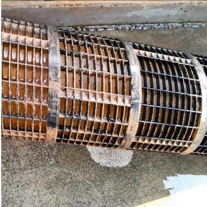
Image – treatment filters full of mud
