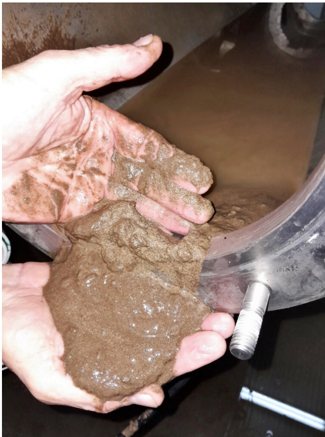
Image – Silt and mud in the water treatment plant at Mossman
