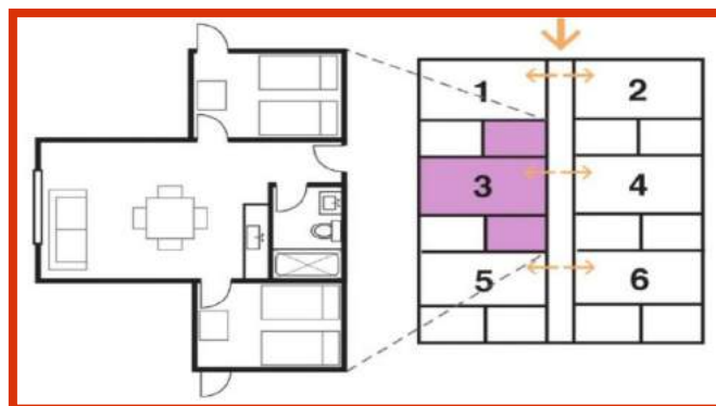
Figure 3: Facility design enabling flexible bed capacity within a communal setting. 16
