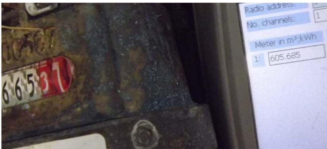
Figure 6 Example of Meter Read Errors due to Reed Switch/MIU Errors (Comparison of mechanical meter totaliser on left with electronic read on right)
