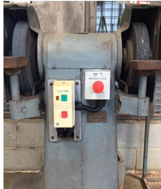
Image: Emergency Stops installed on equipment in the workshop
