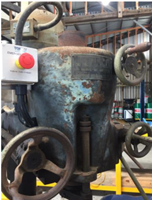
Image: Emergency Stops installed on equipment in the workshop
