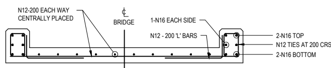
TYPICAL PANEL (TYPES 1, 1A & 1B) REINFORCEMENT SECTION SCALE 1:20
