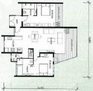
TWO BEDROOM APARTMENT TYPICAL TWO BED APARTMENT AREAS: INTERNAL FLOOR AREA - 51M 2 EXTERNAL FLOOR AREA - 19M 2
