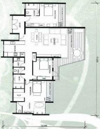
THREE BEDROOM APARTMENT TYPICAL THREE BED APARTMENT AREAS: INTERNAL FLOOR AREA - 73M 2 EXTERNAL FLOOR AREA - 20M 2
