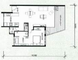
ONE BEDROOM APARTMENT TYPICAL ONE BED APARTMENT AREAS: INTERNAL FLOOR AREA - 47M 2 EXTERNAL FLOOR AREA - 19M 2
