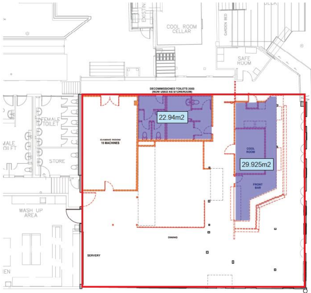
01 Existing Demolition Plan Ground Floor 1:200 @ A3
