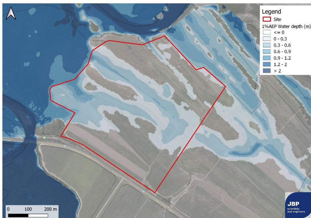
Figure 4-3. Peak flood depth in the 1% AEP flood for existing case
