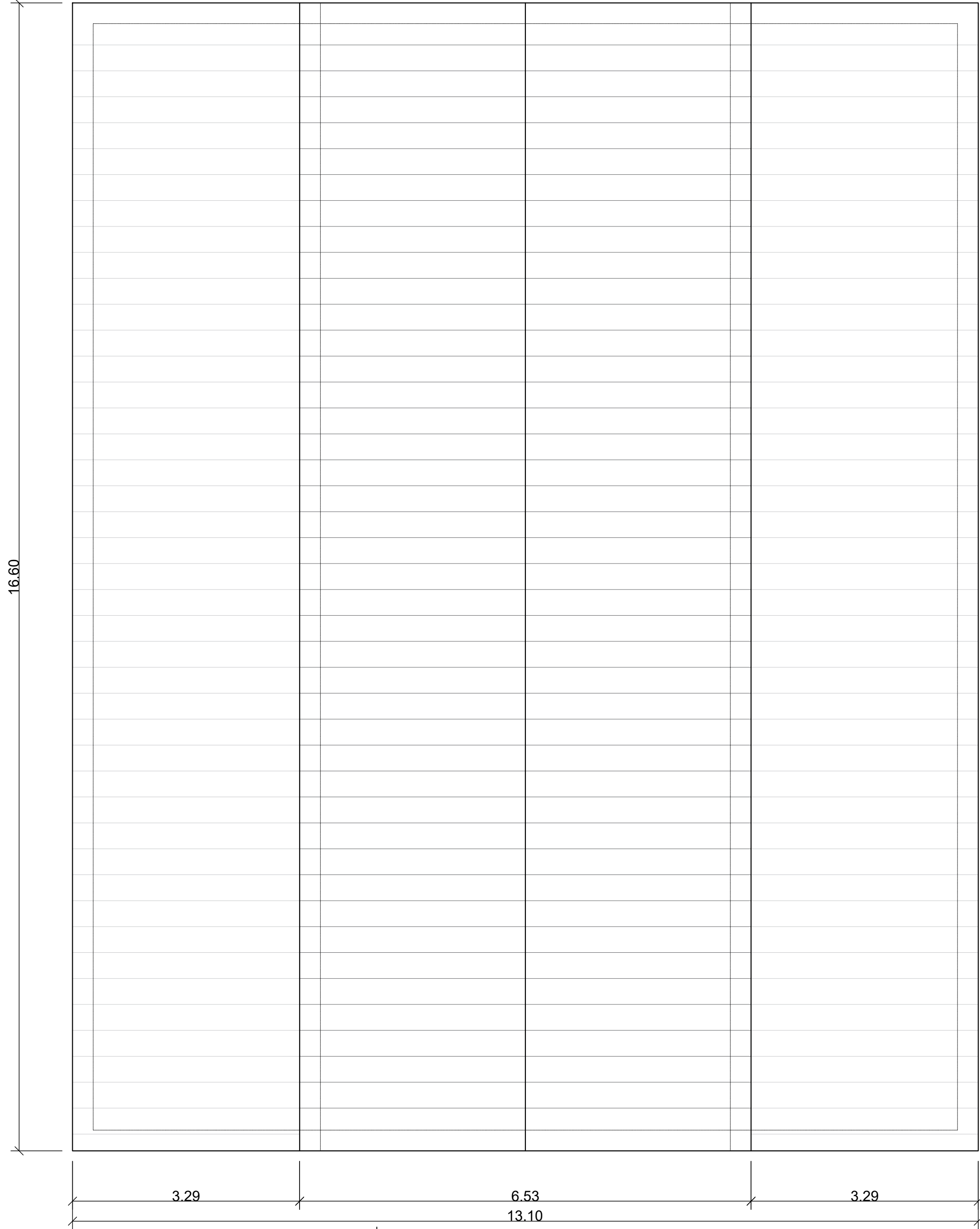
HOBBY SHED ROOF PLAN SCALE: 1:50
