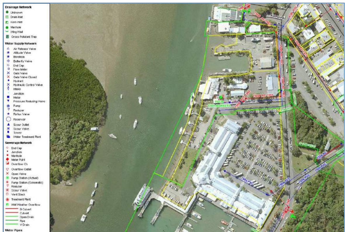
Figure 2: Existing Infrastructure and Services – Water, Sewerage, and Stormwater
