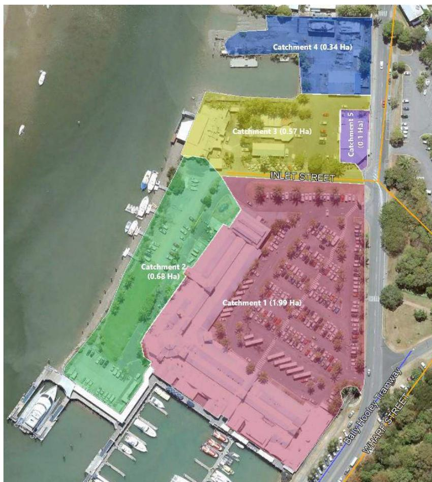
**Figure 2: Existing Stormwater Catchments**
