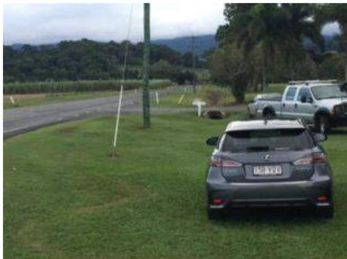
The secondary access/exit point east of the main entry/exit point has restricted sight distance to the east due to current unmaintained vegetation growth which encroaches into the road verge between the two power poles as shown in Photographs 2, 3 & 4.
