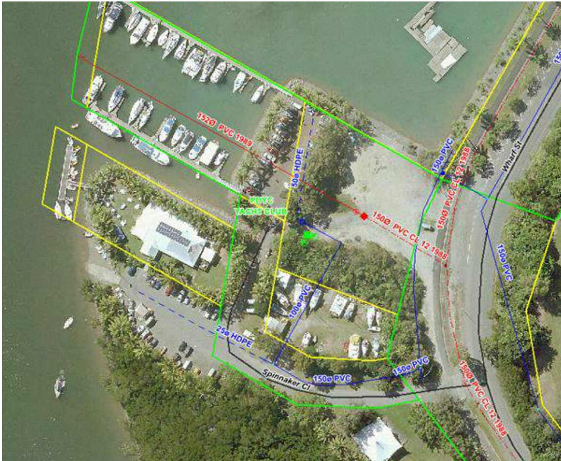
Figure 3: DSC Sewer Main Reticulation
