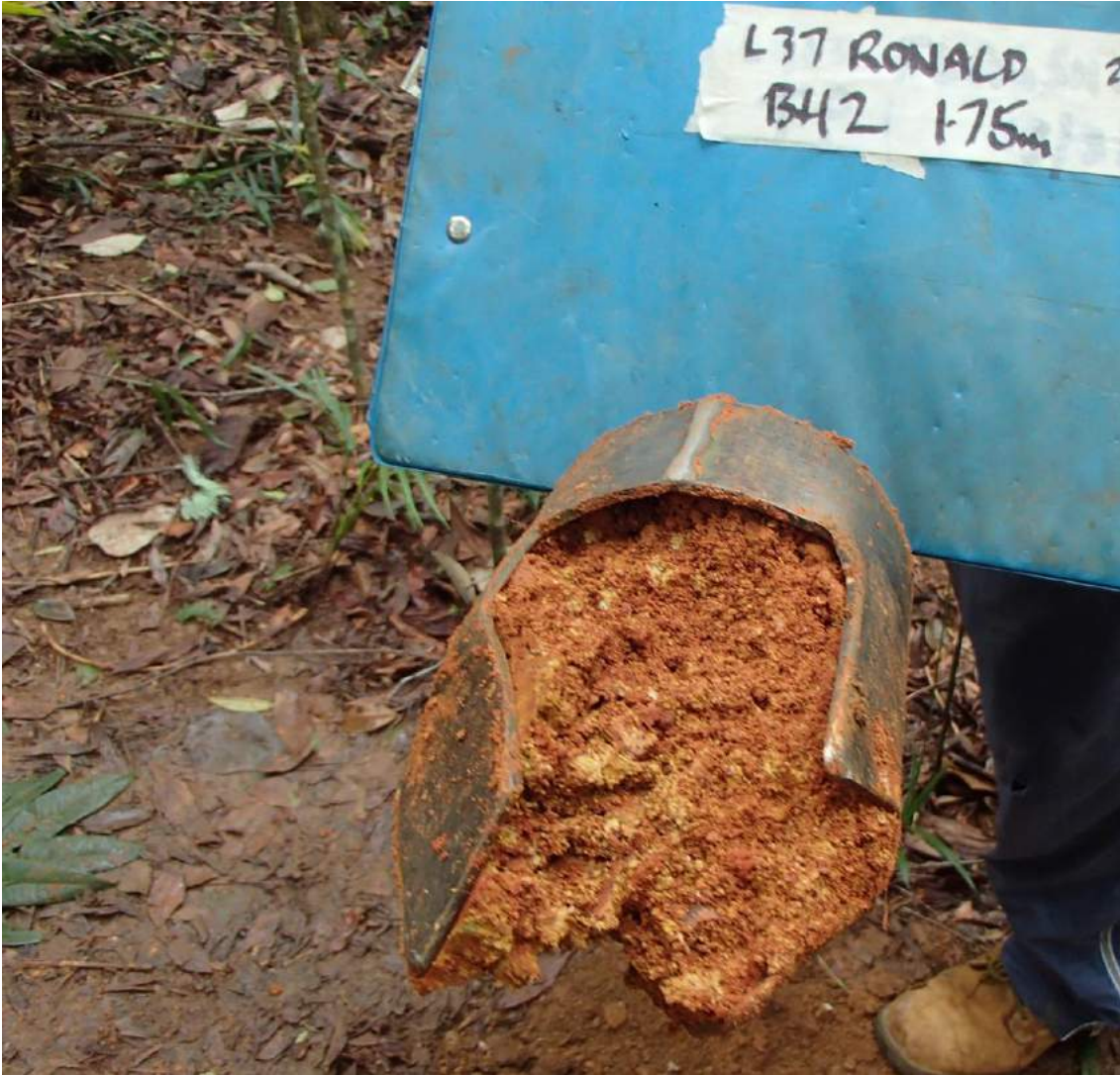
Lot 37 Ronald Road, Forest Creek: BH2, excavated soil @ 1.75m (28/3/18).
