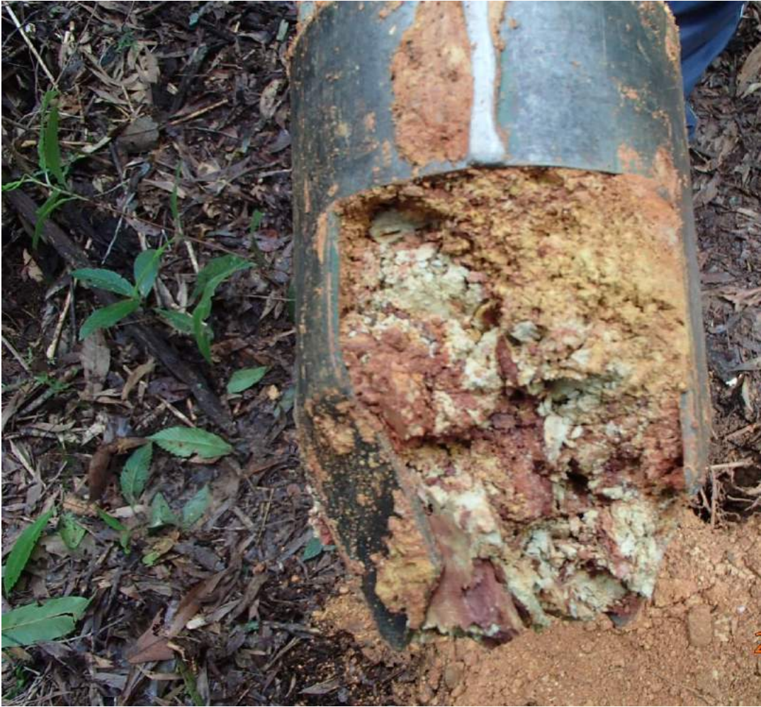
Lot 37 Ronald Road, Forest Creek: BH3, excavated soil @ 1.0m (28/3/18).
