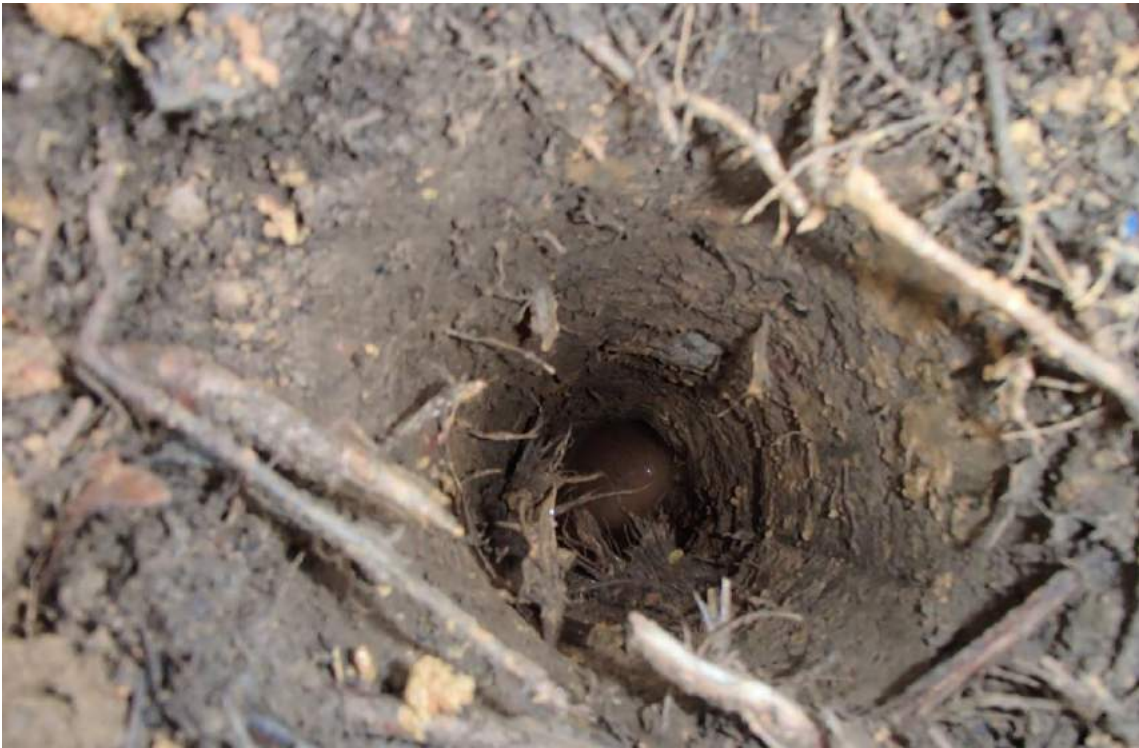
Lot 37 Ronald Road, Forest Creek: BH1, showing groundwater seepage at borehole base (28/3/18).
