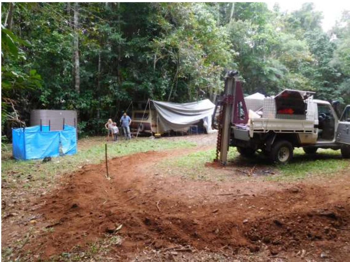
BH1 being sampled at Lot 338 Cape Tribulation Road, Cow Bay
