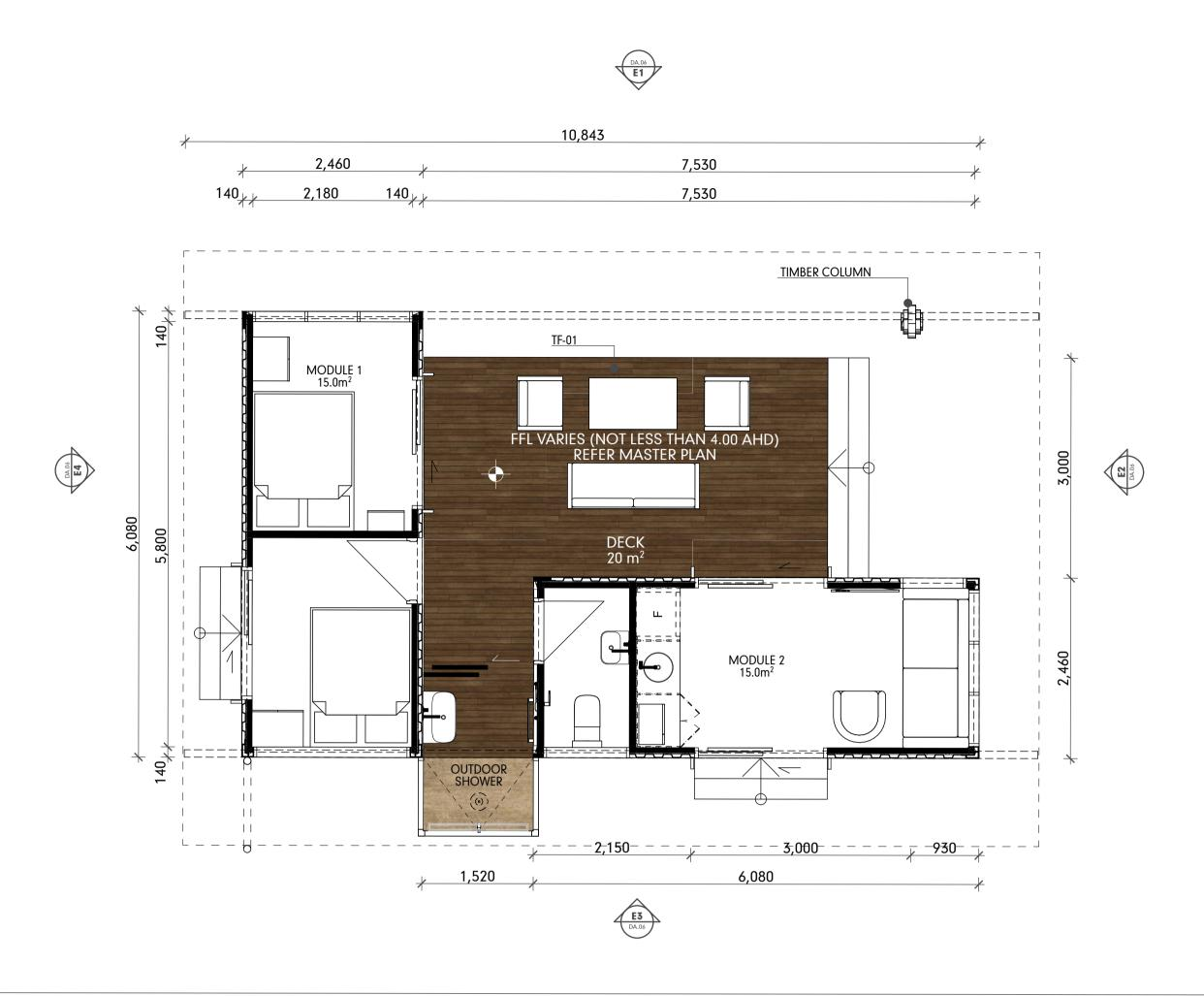
ACCOMMODATION TYPE 1 FLOOR PLAN SCALE1:50
