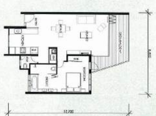
ONE BEDROOM APARTMENT TYPICAL ONE BED APARTMENT VARIANTS: INTERNAL FLOOR AREA - 41M 2 EXTERNAL FLOOR AREA - 14M 2
