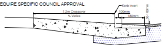
Option 4: 100mm channel at kerb invert NTS
