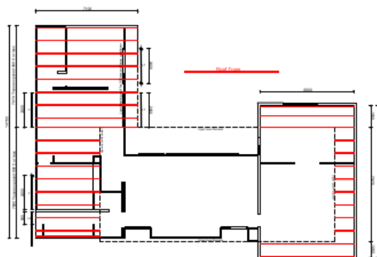
Lower level roof truss / Window lintel Setout
