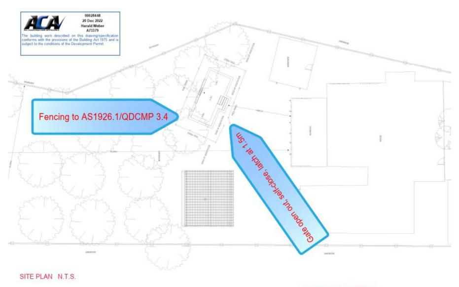
POOL FENCING AND GATES MUST COMPLY WITH AS1926.1, AS1926.2 AND THE BUILDING REGULATION 2006
