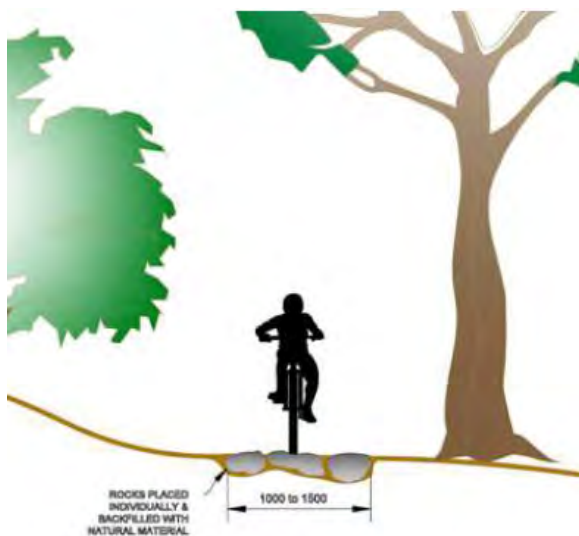
Plate 1 Example of ballast rock used to construct the trail
