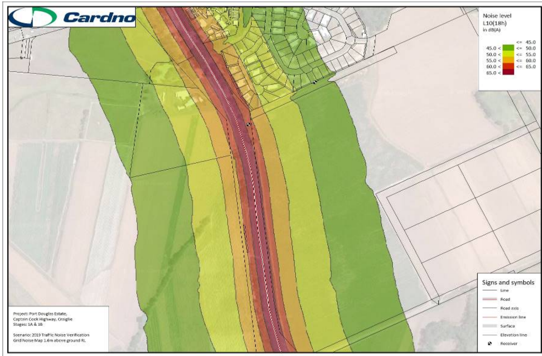
Figure 8-4 Predicted Road Traffic Noise Impact (LA10,18hr) – Existing Year (2019)
