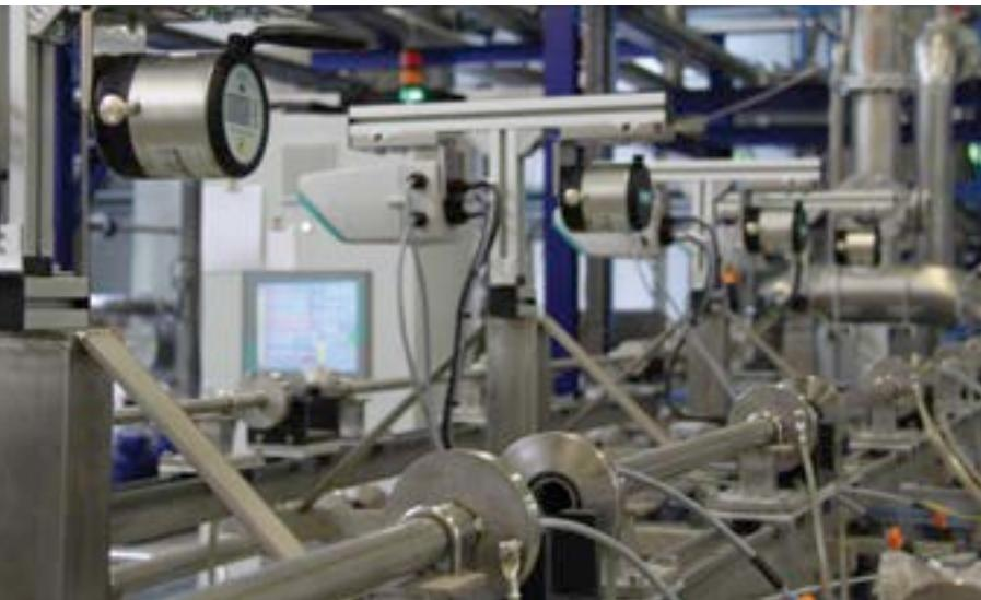
Flowmeter calibration is a vital step in ensuring consistently accurate measurement. All SITRANS F M electromagnetic meters are wet calibrated at Siemens flow facilities with traceable instruments referring directly to the physical unit of measurement according to the International System of Units (SI).
