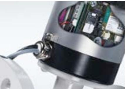
The 3G/UMTS-based wireless communication module collects measurement data from meters anywhere in the world covered by the 3G/2G network. Alarms from the MAG 8000 are sent immediately to the customer once an alarm signal is detected by the module at a minimum sample interval of 1 minute.
