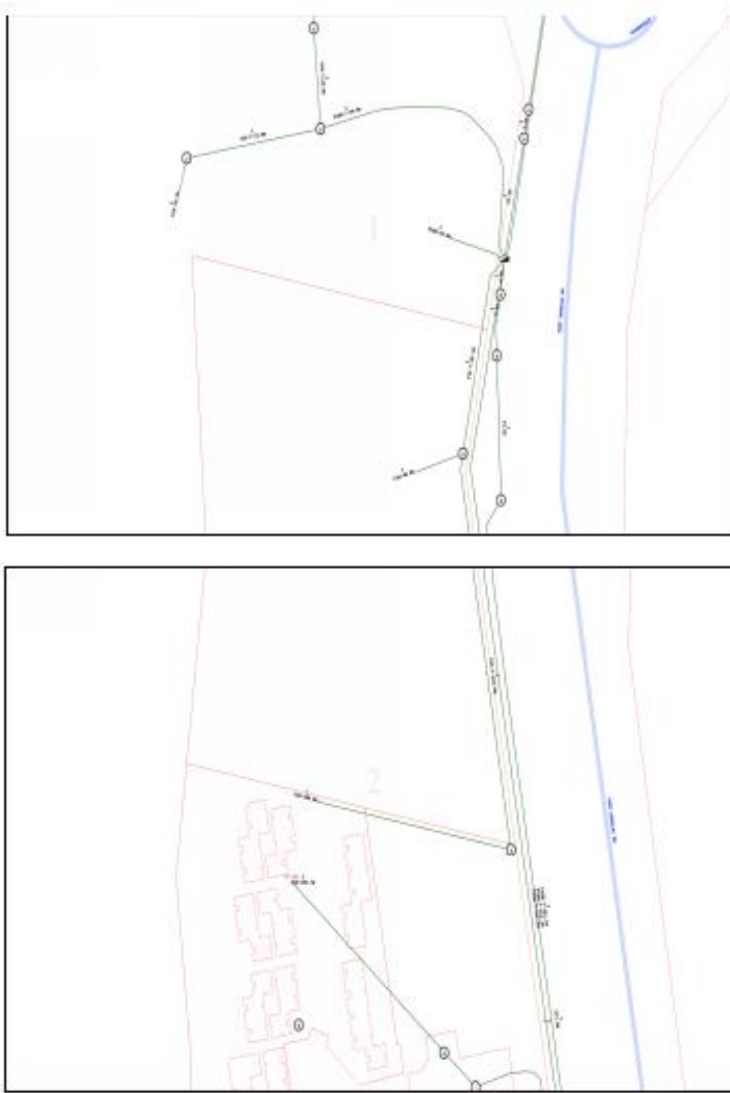
Figure 7 – Extract of NBN Network – Green Indicates existing conduit network
