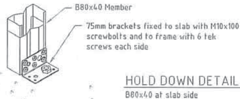
HOLD DOWN DETAIL 2 B80x40 at slab side
