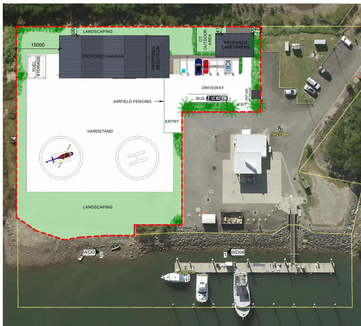
Figure 4 – Proposed Helipad Landing Facility layout
