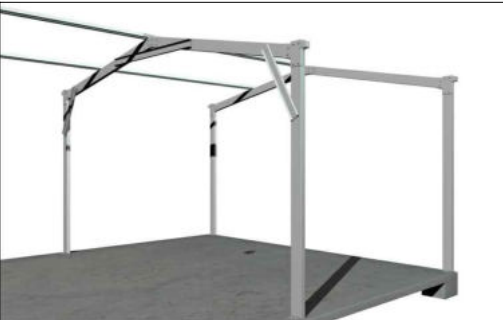
2A FIRST & SECOND PORTAL FRAME ASSEMBLY 1 REFER 2C FOR TEMPORARY BRACING LOCATION
