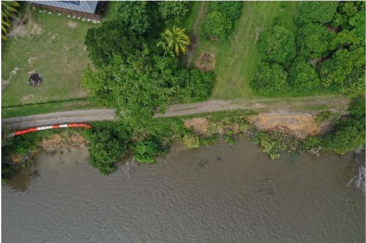
Figure 6. Photograph of erosion threatening the access road/esplanade at site DR-4
