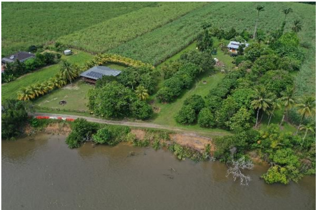
Figure 5. Photograph of erosion threatening the access road/esplanade at site DR-4
