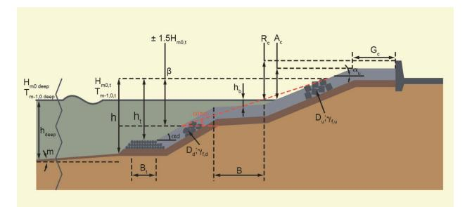
Figure 5: Schematisation of the structure, including the parameters required to run the NN tool (Figure 4.16, EurOtop 2018)
