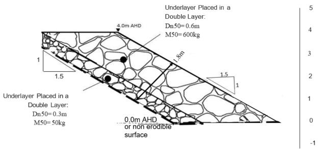
Figure 4: Typical revetment wall design cross-section
