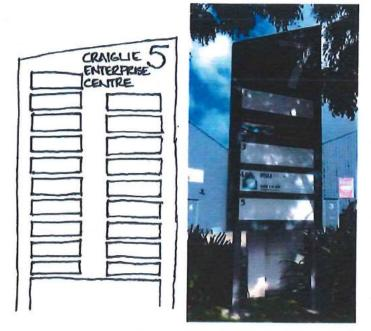
Please note the final dimensions (width in particular) for the sign will be confirmed with the sign designer / installer. At this stage, noting the maximum height of sheds is 5.1m, the height of the sign will be limited to this, although the width may be altered to ensure the sign area available for each tenancy is at least 30cm in height, and potentially 1m or so in width.
