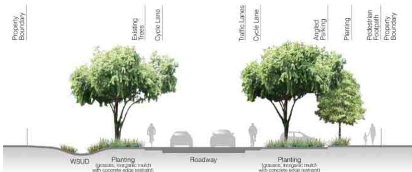
Typical Cross Section - Warner Street (between Owen and Grant Streets)
