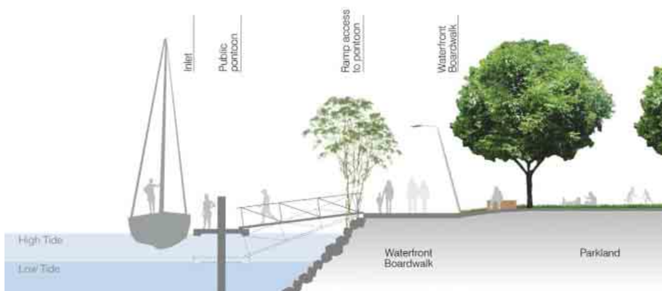
Typical Cross Section - Mooring Pontoon and Boardwalk
