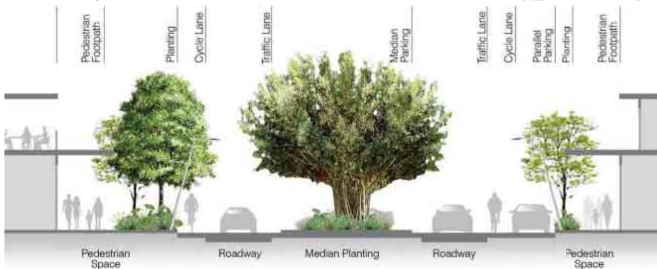
Typical Cross Section - Macrossan Street
