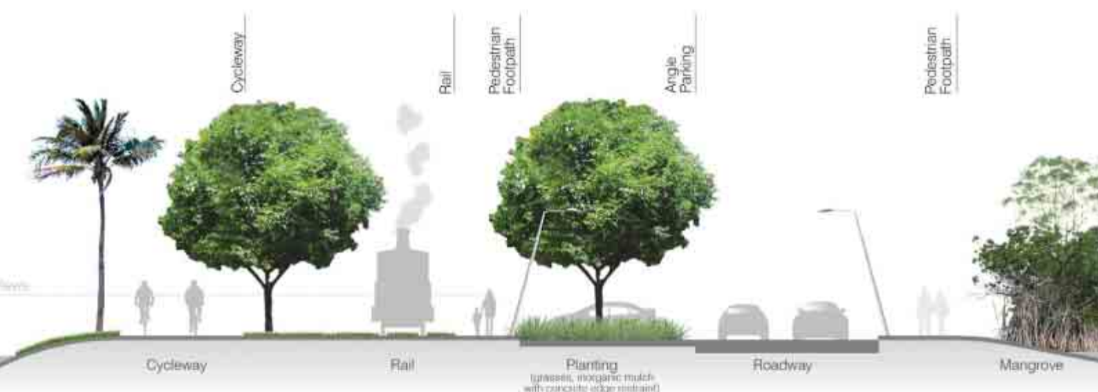
Typical Cross Section - Wharf Street (between Port and Mowbray Streets)
